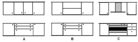
In addition, there is also a range of horizontal "lift-up" units – see website for details and sizes. In general you should try to match the width of the base units with the wall units, ie put a 2" wall unit over a 2" base unit etc, or a 3" unit over two adjacent 1½" ones. Another example is to put two 3" horizontal wall units over three 2" base units.
