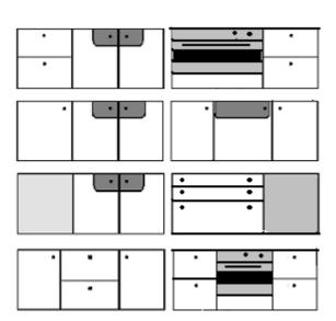
The 5" unit is one of the most flexible. It is equivalent to one 2" and two  $1\frac{1}{2}$ " spaces, or one 2" and one 3" space. Hence the unit can be used as a corner unit, left or right (order corner panels), with either wide drawers, or one door  $(1\frac{1}{2}$ ") and one set of drawers  $(1\frac{1}{2}$ ") or a two-door cupboard, into which can place the sink if you wish (order two  $1\frac{1}{2}$ " doors).
