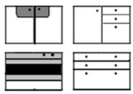
The 3" unit can be used with two  $1\frac{1}{2}$ " doors or one door and one  $1\frac{1}{2}$ " set of drawer fronts (note panelled drawers consist of two equal drawers). It can also be used as a wide drawer unit, or an oven. You can also use it as the base for any of the sinks (except the Butler sink).
