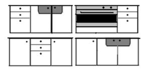
The  $4\frac{1}{2}$ " unit can be used as a three-door unit (three  $1\frac{1}{2}$ " doors) or you can add one or more sets of drawers ( $1\frac{1}{2}$ "). If you place these to one side, you can use the remaining double cupboard as a sink unit. Alternatively you can place the drawers in the centre. You can also use two sections for the wide oven or a set of wide drawers (see 3" unit).
