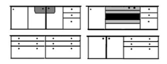
The 6" unit is the equivalent of four  $1\frac{1}{2}$ ", two 3", or one 3" unit and two  $1\frac{1}{2}$ " units. You can place the sink in any section with two adjacent  $1\frac{1}{2}$ " doors. One double section can be used for the wide oven, and one or both for wide drawers.
